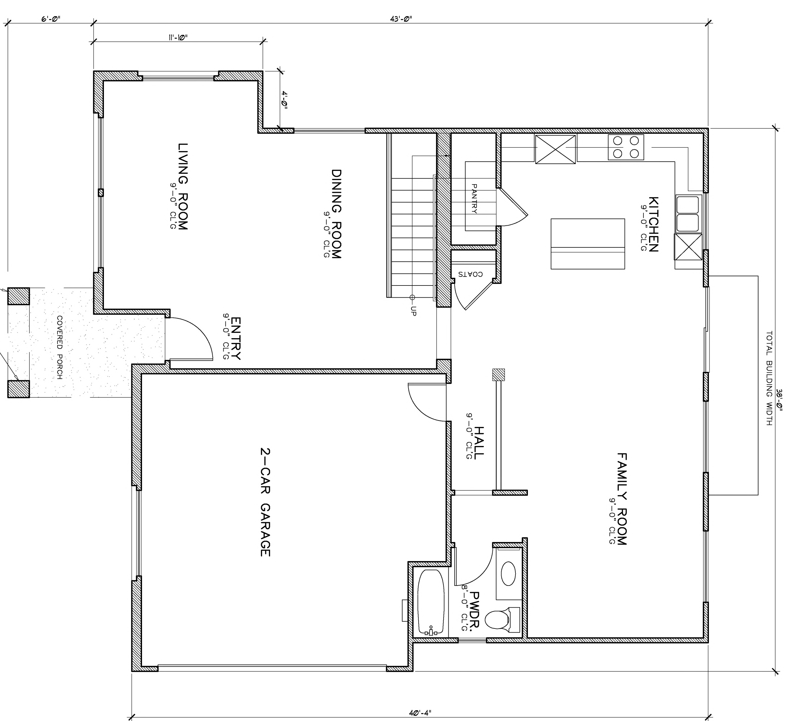
FIRST FLOOR PLAN SCALE: 1/4" = 1'-0"
